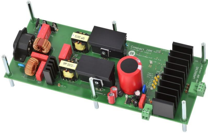
1kW motor inverter with PFC
